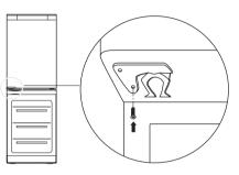
Carefully slide the fridge compartment door onto the top bearing pivot and close.
